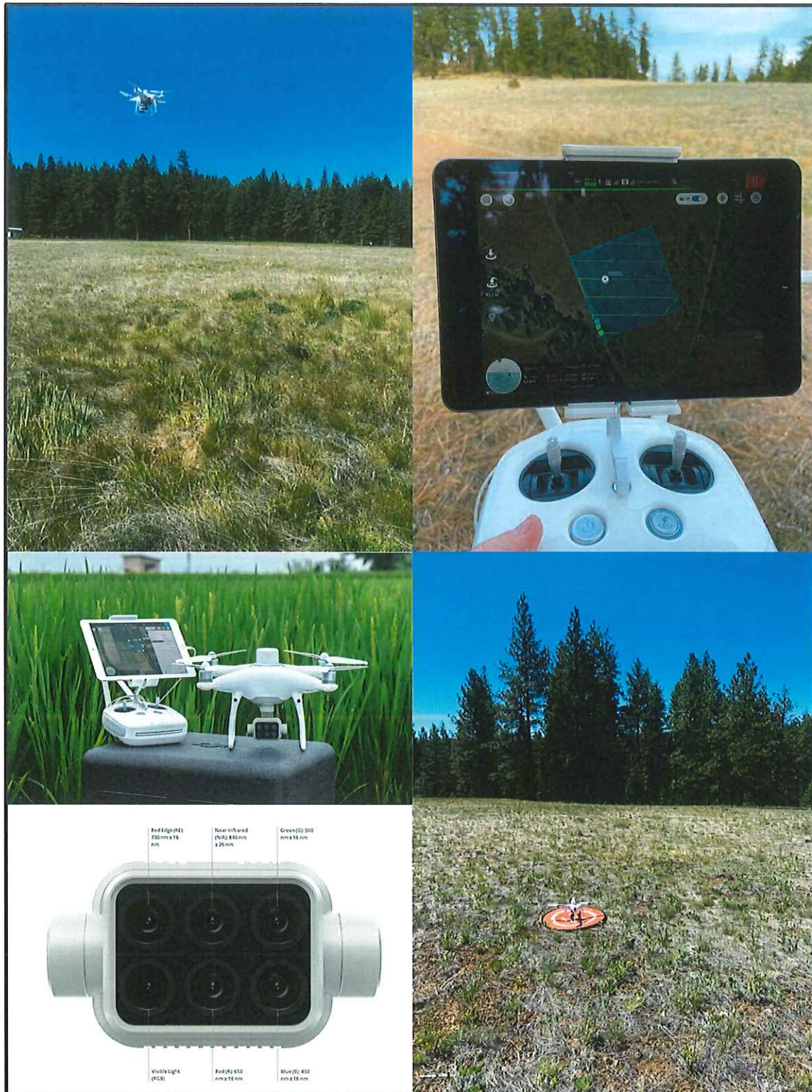
Figure 1. We utilized a DJI Phantom P4 Multispectral drone. This drone has a multispectral camera which allows us to capture regular (RGB) images, as well as Blue, Green, Red, Red Edge, and Near Infrared bands, which allows us to gain better insight on plant health. Flights are planned and flown using a basic iPad mini and controller.
