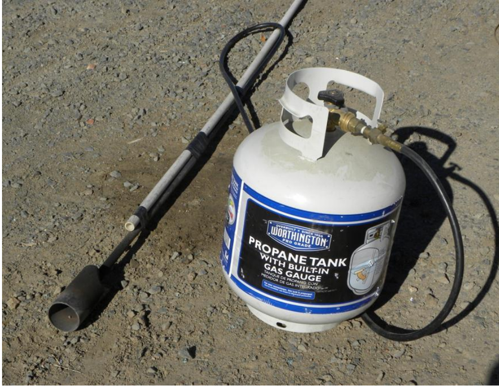
Fig. 1. A photo of the handheld propane flamer used for flaming peppermint plants in the microplot trial. An extended torch was attached to a 5-gallon propane tank.
