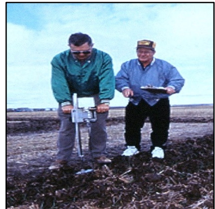
Dr. Clyde Douglas and Paul Rasmussen using a soil penetrometer to determine the strength of a silica-cemented layer
