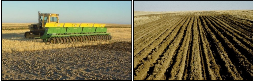
John Deere HZ deep-furrow seed drill and depressed furrows in cultivated fallow
