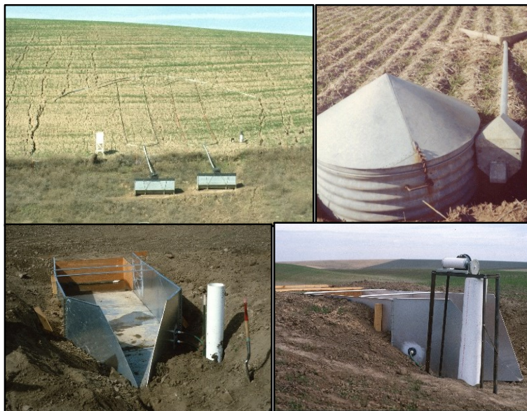
Hillslope configuration for erosion research in Gilliam, Wasco and Sherman counties, and three types of flumes for measuring or collecting runoff water and soil
