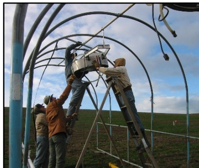
Constructing a simulated rainfall structure over a field of winter wheat
