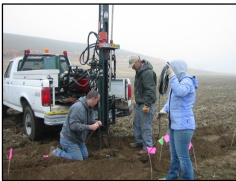
David Robertson and Dr. Don Wysocki using a soil probe to collect samples to determine soil water content
