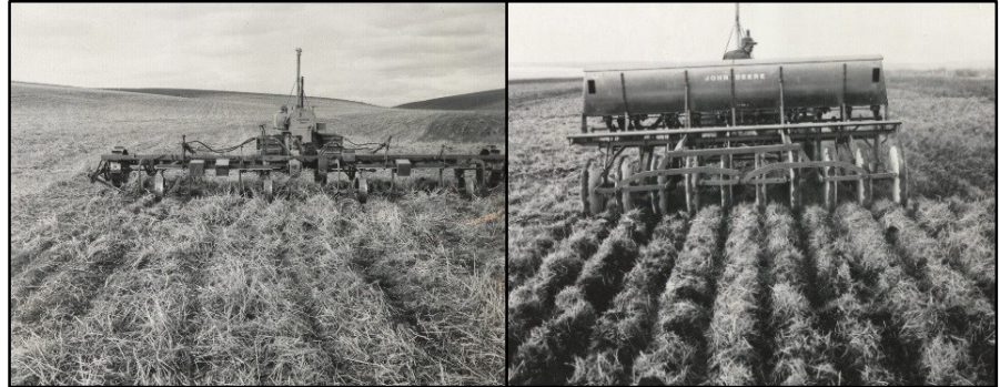
Successfully rod weeding and planting deeply into heavy residue using a John Deere HZ deep-furrow drill at the King Pilot Farm
