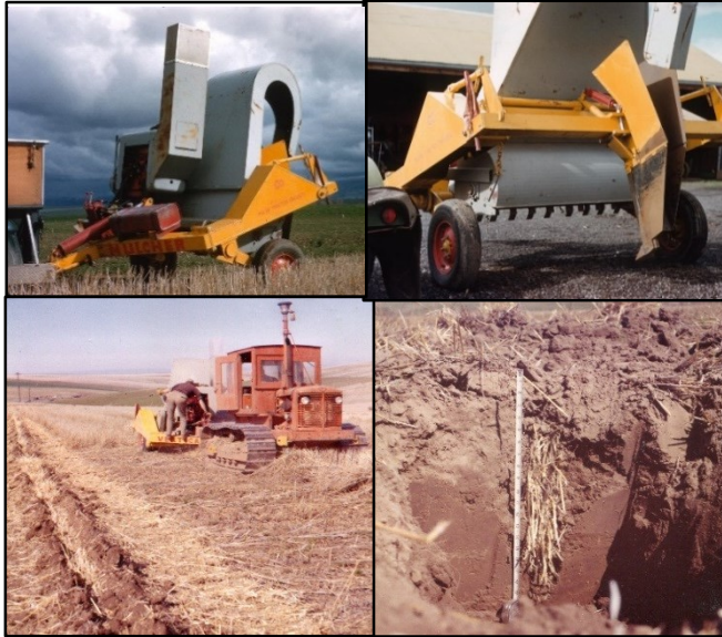
Vertical mulching equipment and views of the field surface and a straw-filled trench
