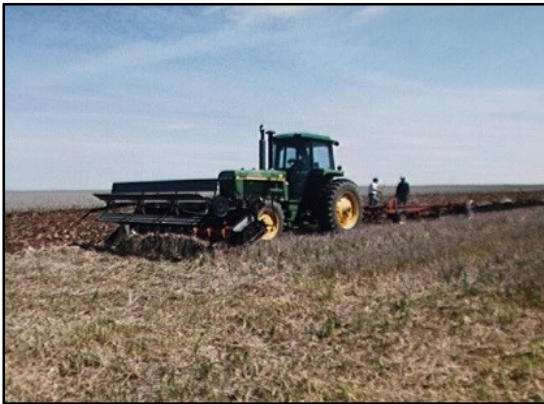
Mow-plow system. Stubble cut with a header is blown sideways onto freshly plowed soil. The moldboard plow behind the tractor inverts remaining stubble.
