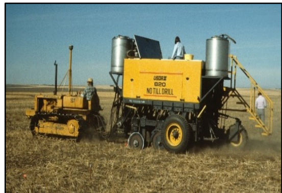
Yielder No-till Drill: an early version of a drill designed for planting into non-cultivated soil
