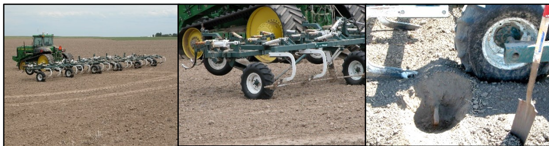
A modern rod-weeder with raised rod (left and center), and at operational 4-inch depth (right)
