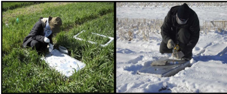
Gas-collection chambers for measuring emissions of carbon dioxide, nitrous oxide and methane
