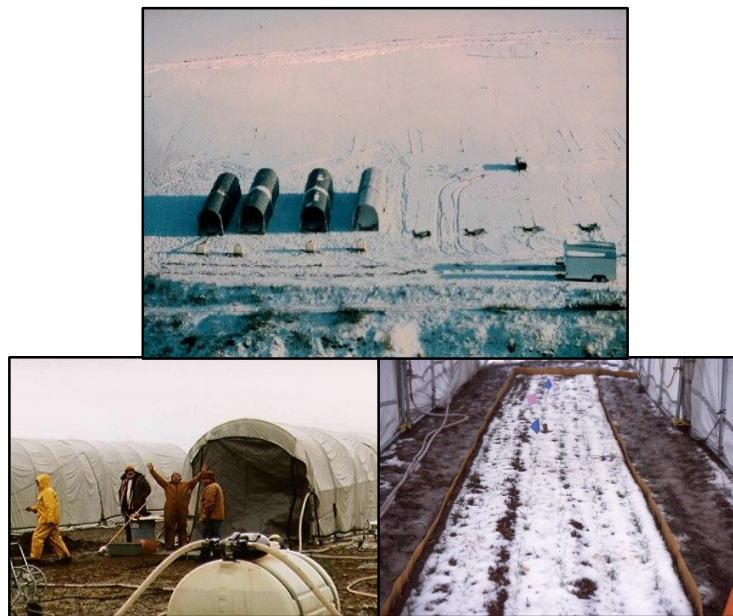
Simulated rainfall used to compare runoff and erosion from frozen soil on hillslopes cultivated using three plow-based tillage systems; mow-plow, moldboard and chisel plow.
