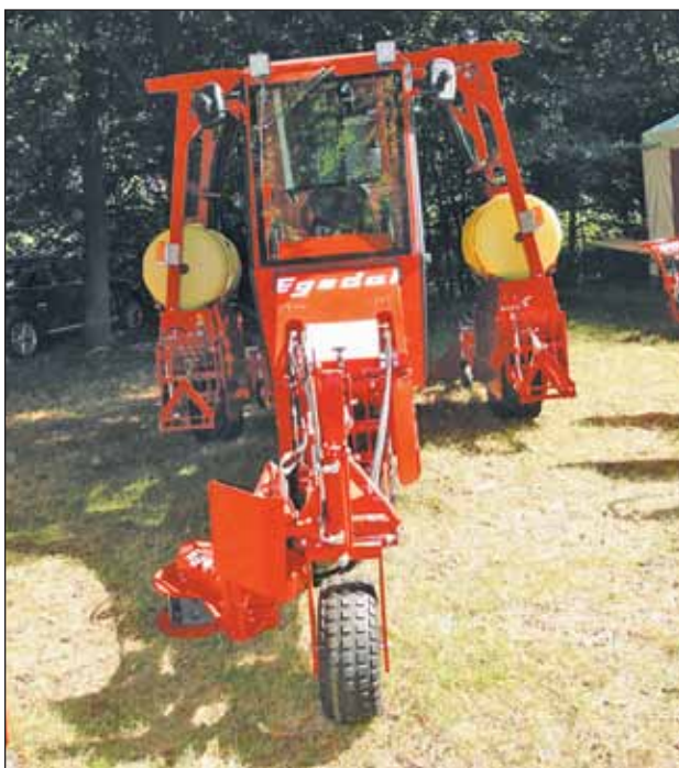
Shiny new multi-row machine set up to spray and prune the base of the trees.
